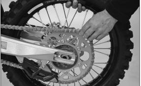
The rear wheel is remounted in the reverse order. Before tightening the collar nut to 80 Nm (60 ft.lb), push the rear wheel forwards so that the chain tensioners lie on the tension screws.
